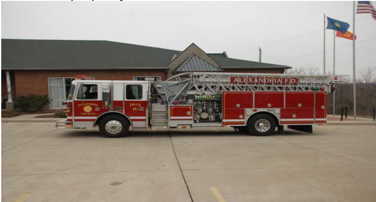
Truck Company 110 1994 Sutphen 75+ Aerial Ladder 1500 GPM Pump Capability
