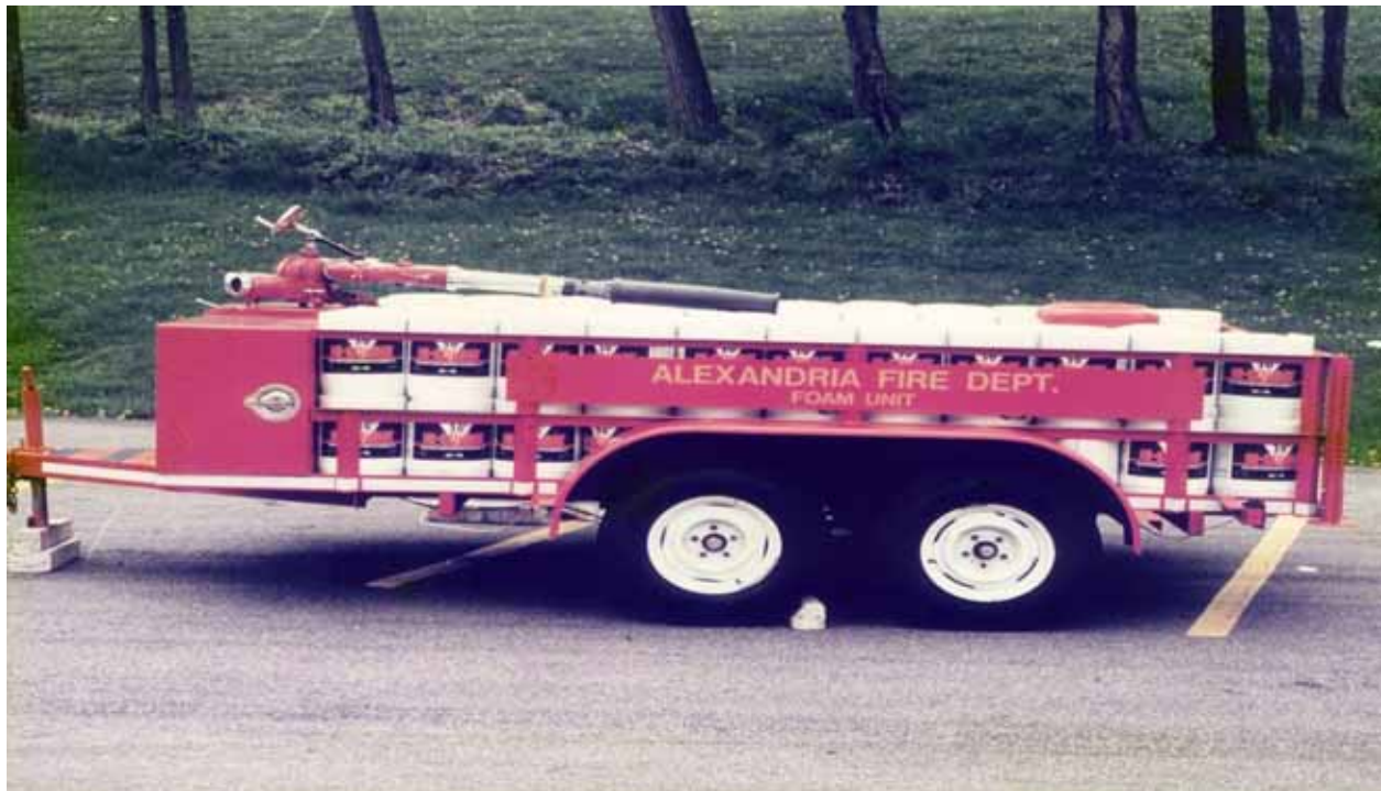
Foam Unit Unit 136 75-5 gallon buckets of foam
